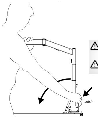
Press down on the latch. Hold the hoist jib when the latch loosens so that it does not fall uncontrollably to the ground.
