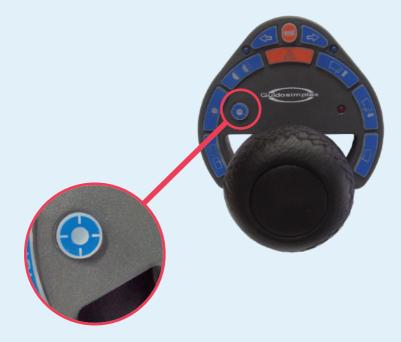
When this function is no longer required the switch must be returned to the off position.
