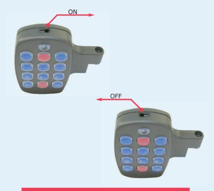
When this function is no longer required the switch must be returned to the off position.
