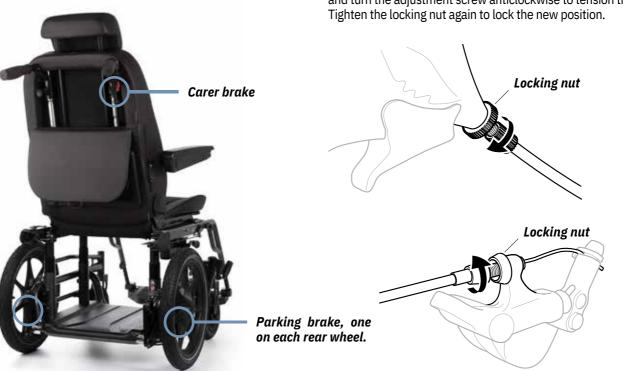
If the brakes are not engaging properly, slacken the locking nut and turn the adjustment screw anticlockwise to tension the cable. Tighten the locking nut again to lock the new position.
