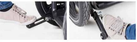
Use the anti-tipping device if necessary. Press the top of the support to fold it down. Press the black catch up or down to fold the support up again.
