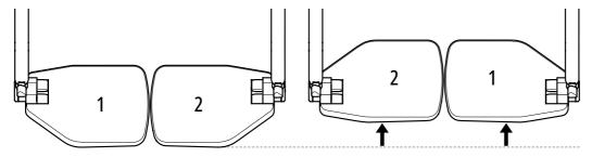
If necessary, move the position of the foot plates so that they are closer to the user.
