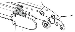
**3** Press down the release lever. Slide the seat all the way in and secure it on the chassis with a firm press.
